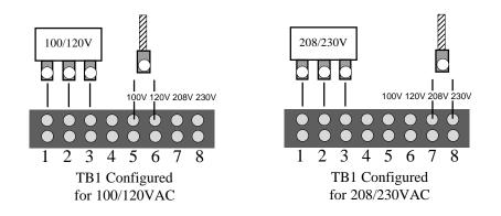
Move "Voltage Selector Cable" to the corresponding input voltage terminal of TB1 for 100V, 120V, 208V, or 230V.
