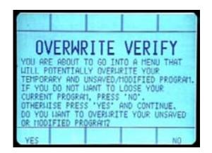
If 'NO' is pressed, the screen will return to the WELD ORBITAL screen. If 'YES' is pressed, the screen will change to RECALL USER MEMORY.
