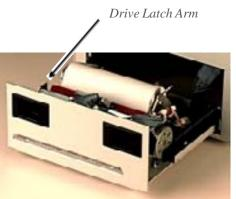
Insert roll of paper between pins and spin backward to pull up any extra slack in the paper. Engage the Drive Latch Arm upward to secure the Printer Drive Mechanism.
