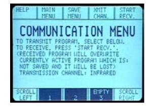
It is from this screen that weld procedures can be transferred from one CobraTig<sup>™</sup> 150 unit to another. There are two paths available for transmission: IR (Infra Red) and Wired Cable. The IR method works much like a TV remote, just have the two units facing each other at a distance up to 10 feet and commence transmitting. While the Wired Cable is a cable hookup between the units' RS232 transmission ports on the rear panels.
