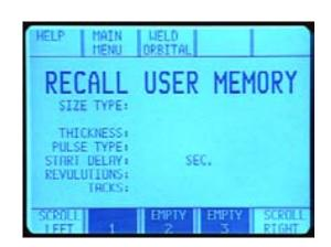
Press the RECALL PROGRAM in order to access the library of operator saved weld procedures.
