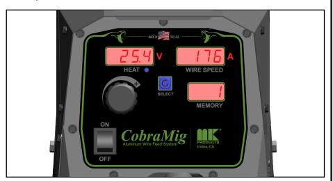
Note: Once arc is established during welding, actual welding Voltage and Amps will be live and displayed on the user interface. After welding, actual Volts and Amps will remain displayed for three seconds before resetting back to Reference Voltage and Wire Speed. See example above.
