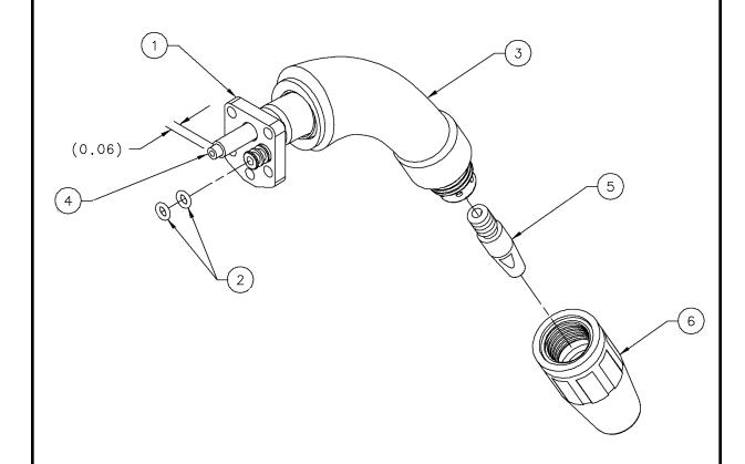
\*Apply silicone lubricant to item 2 before installing.
