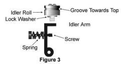
NOTE: Lock washer must be under idler roll or it will not turn freely.
