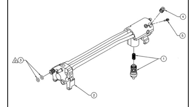
APPLY SILICONE LUBRICANT TO O-RING BEFORE INSTALLING.
