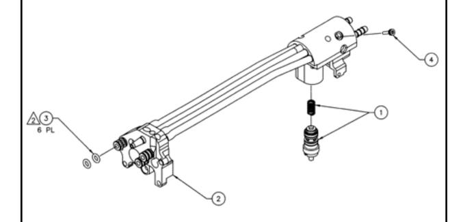
APPLY SILICONE LUBRICANT TO O-RING BEFORE INSTALLING.
