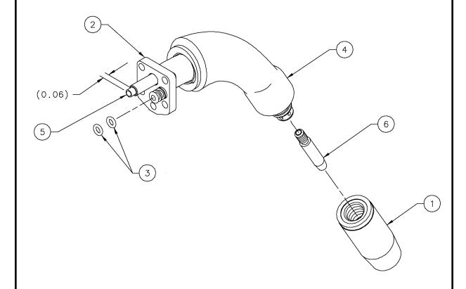
\*Apply silicone lubricant to item 3 before installing.
