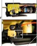
Screw adjusted out of trigger, pre-setting the micro-switch lever for shorter motion sensitivty.
